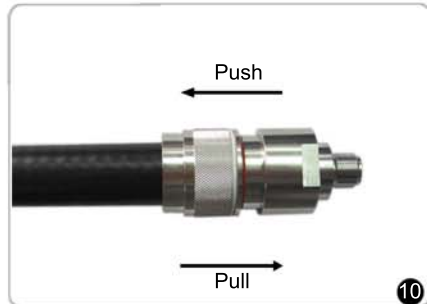
Push the connector onto the cable. Then pull the connector to make sure the connector can not be pulled off.
